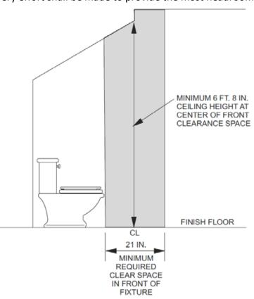
wall or other side barrier (tub). The clear space in front of the water closet shall be at least 21". Water closets must be sealed to the floor with appropriate caulks.
