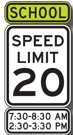
MUTCD sign example of a school zone sign assembly. Photo credit: FHWA, 2009
