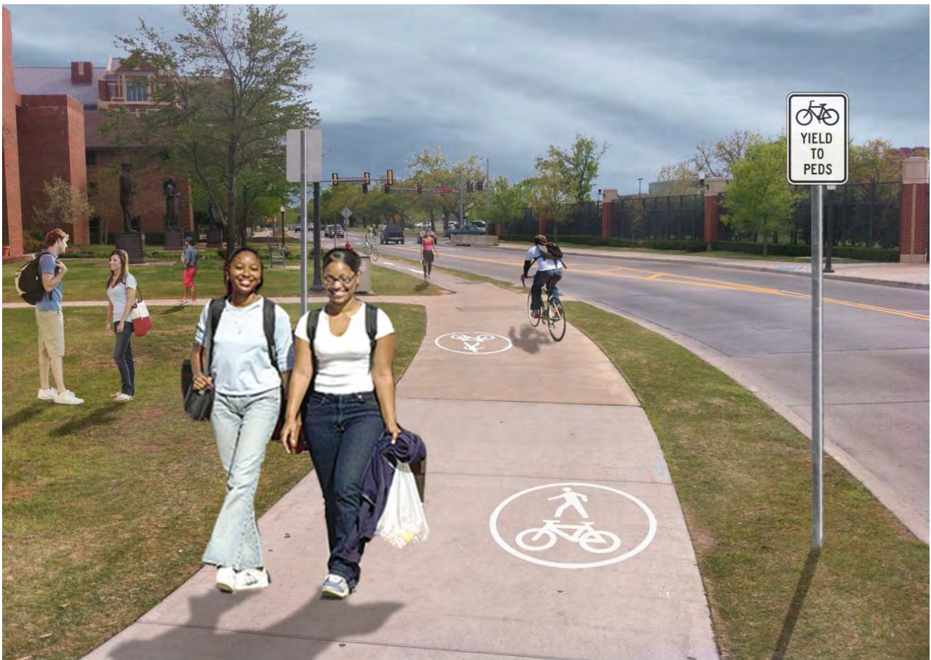
Figure 109: This sidepath example includes pavement markings to indicate that both pedestrians and bicyclists are permitted to use the facility.
