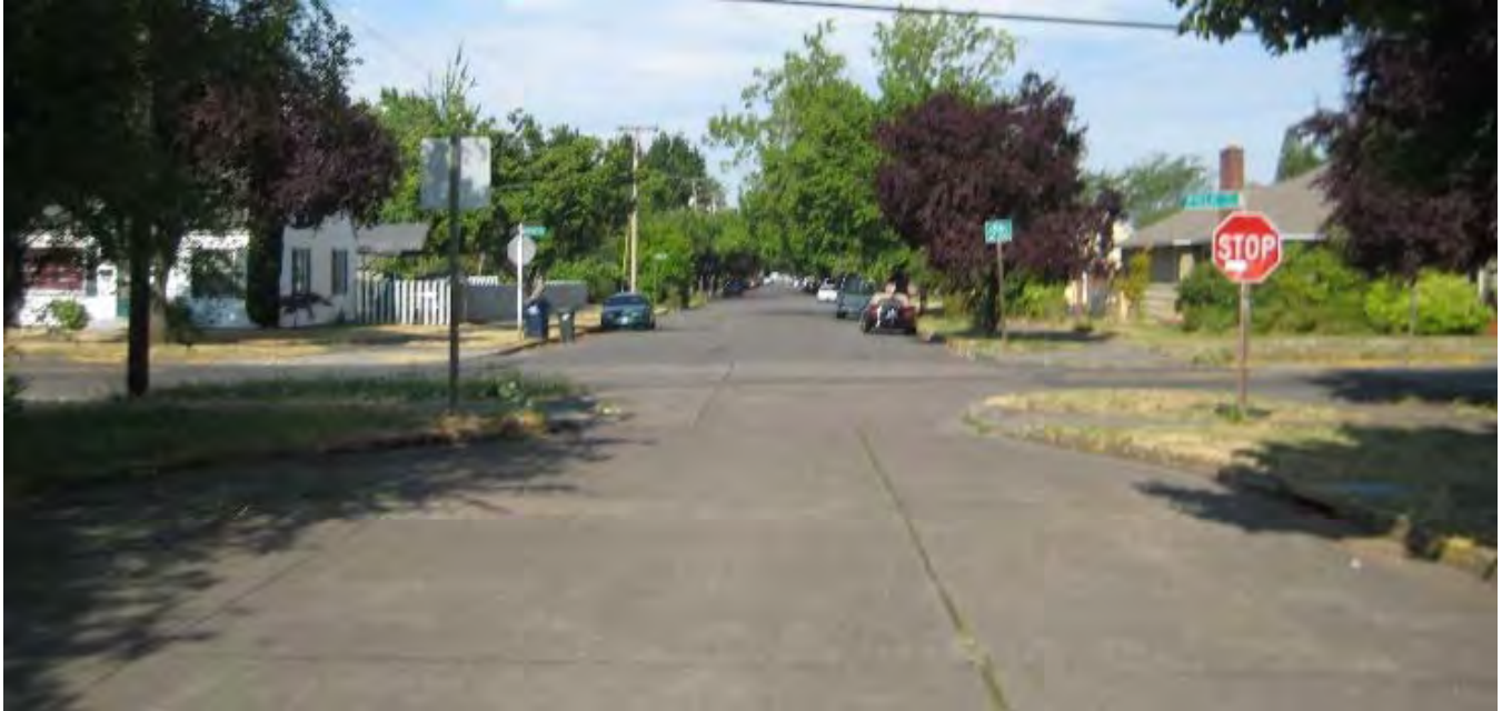
Figure 63: A neckdown reduces the street width at an intersection, decreasing pedestrian crossing widths, limiting turning radii, and slowing down motor vehicle speeds.
