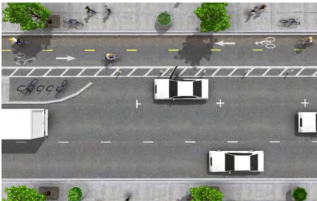
Figure 55: This cycle track diagram incorporates raised bollards to separate bicyclists from motor vehicles.
