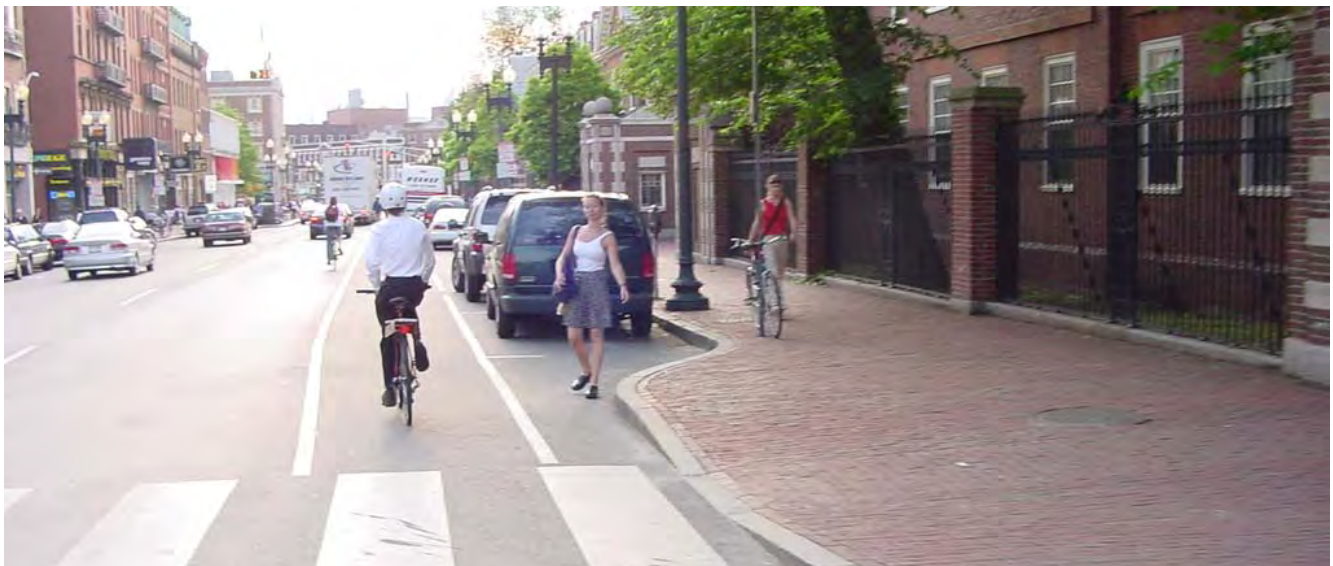
Figure 110: When designed properly, bicycle lanes separate bicyclists from motor vehicle traffic while also protecting bicyclists from the opening doors of parked cars.
