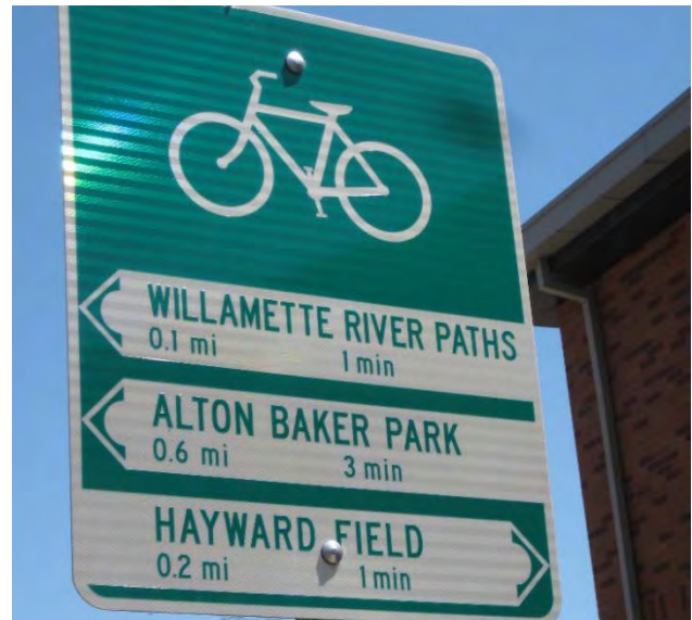
Figure 88: Decisions signs are used in advance of intersecting bike routes.
