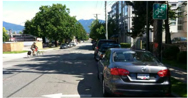
Figure 87: Turn signs are placed in advance of a turn in the bike route network.
