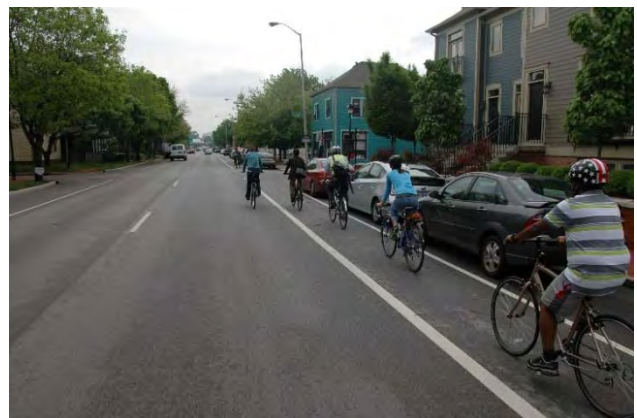
Figure 48: Bicycle lanes provide dedicated space on the roadway for bicyclists.
