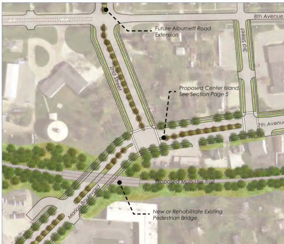
Figure 3: Conceptual Plans for the West End Corridor propose a renovation or replacement of the railroad bridge over Marion Boulevard for bicycle and pedestrian use.
