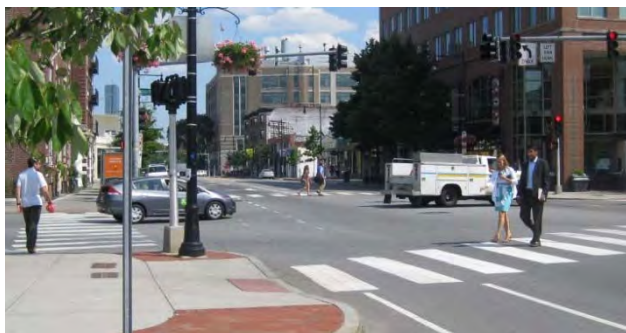
Figure 33: Bulb-outs increase motorists' visibility of pedestrians while also reducing turning speeds.
