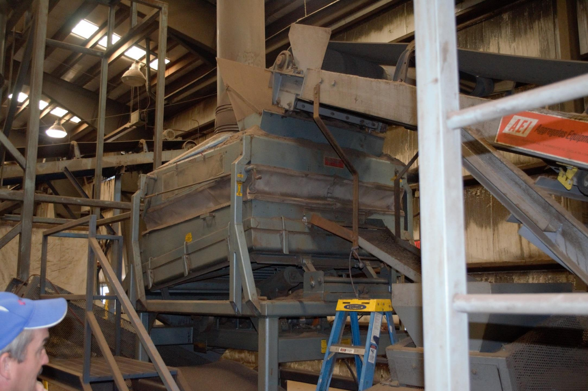
Air Classifier- Utilized to screen compost
