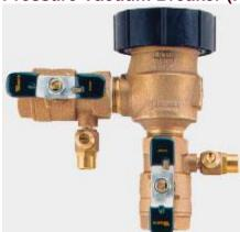
A testable assembly containing an independent, internally loaded check valve and an independent, loaded air inlet valve located on the discharge side of the check valve. This assembly is designed to protect against a non-health or health hazard under back-siphon conditions only.
