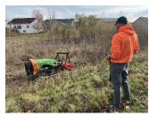
on. The unit can mow up to a 60-degree slope, and mulches trees up to 6 inches in diameter.
