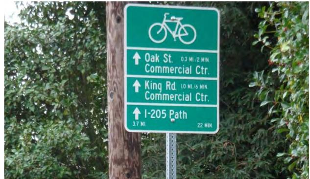
Figure 86: An example of a typical confirmation sign.
