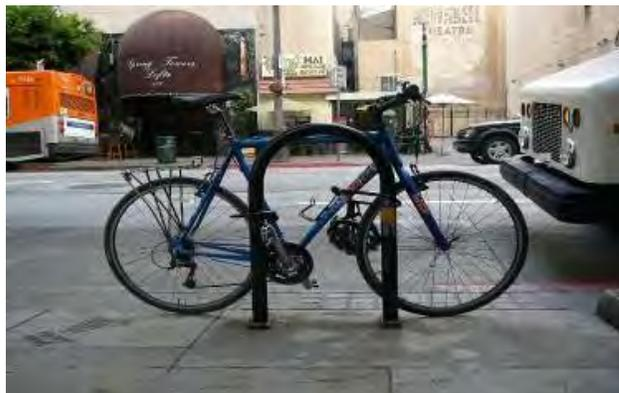
Figure 118: Simple staple racks, or "inverted U" racks, provide cyclists with the necessary security and stability to properly lock their bicycles.
