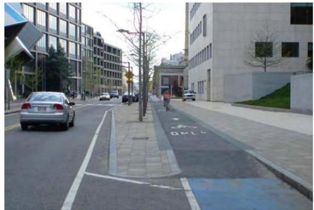
Figure 52: A raised cycle track in Cambridge, Massachusetts.
